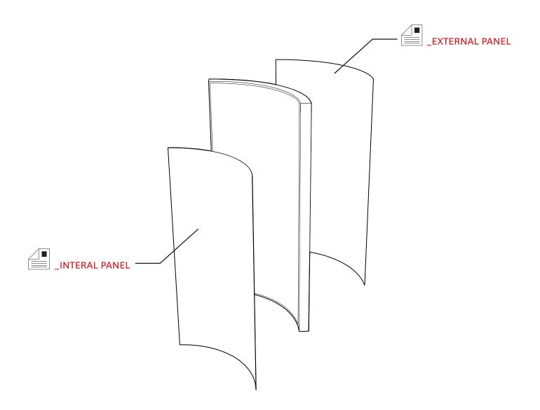
You need to remember that due to the curved shape of the frame the internal and external panels have different widths.
